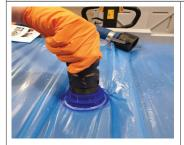
Without further unfolding the liner remove the white cap and insert the 2" cam adaptor to the inlet port.
