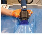
To this attach the appropriate filling adapter for the filling source (the rigid fill hose provided shown here).
