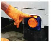
Attach the open/close handle to the outlet liner valve spindle. The valve opens clockwise
