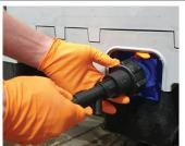
Attach the required outlet fitment and open the liner valve. Remove key if required.
